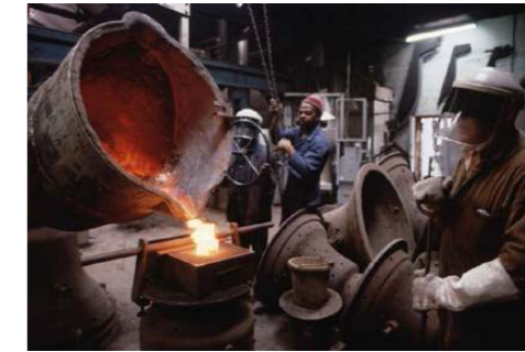
Casting bells at Whitechapel in 1997 with the traditional loam and greensand method
