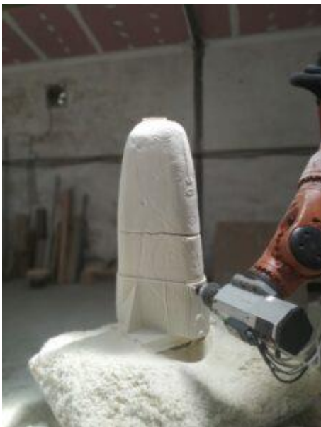
Reunited Ntitogo monolith being CNC-milled, using computer controlled machining tools.
