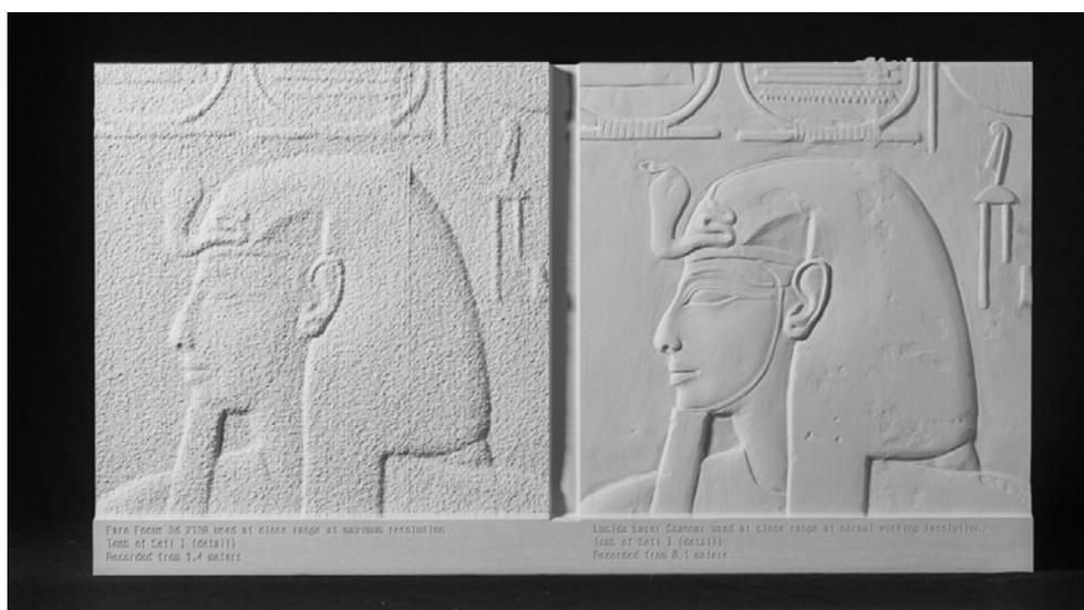
*Maximum resolution recorded with the Faro scanner working at its minimum distance (left image) and the same section of the tomb of Seti I recorded with a Lucida scanner under normal working conditions (right image).*
