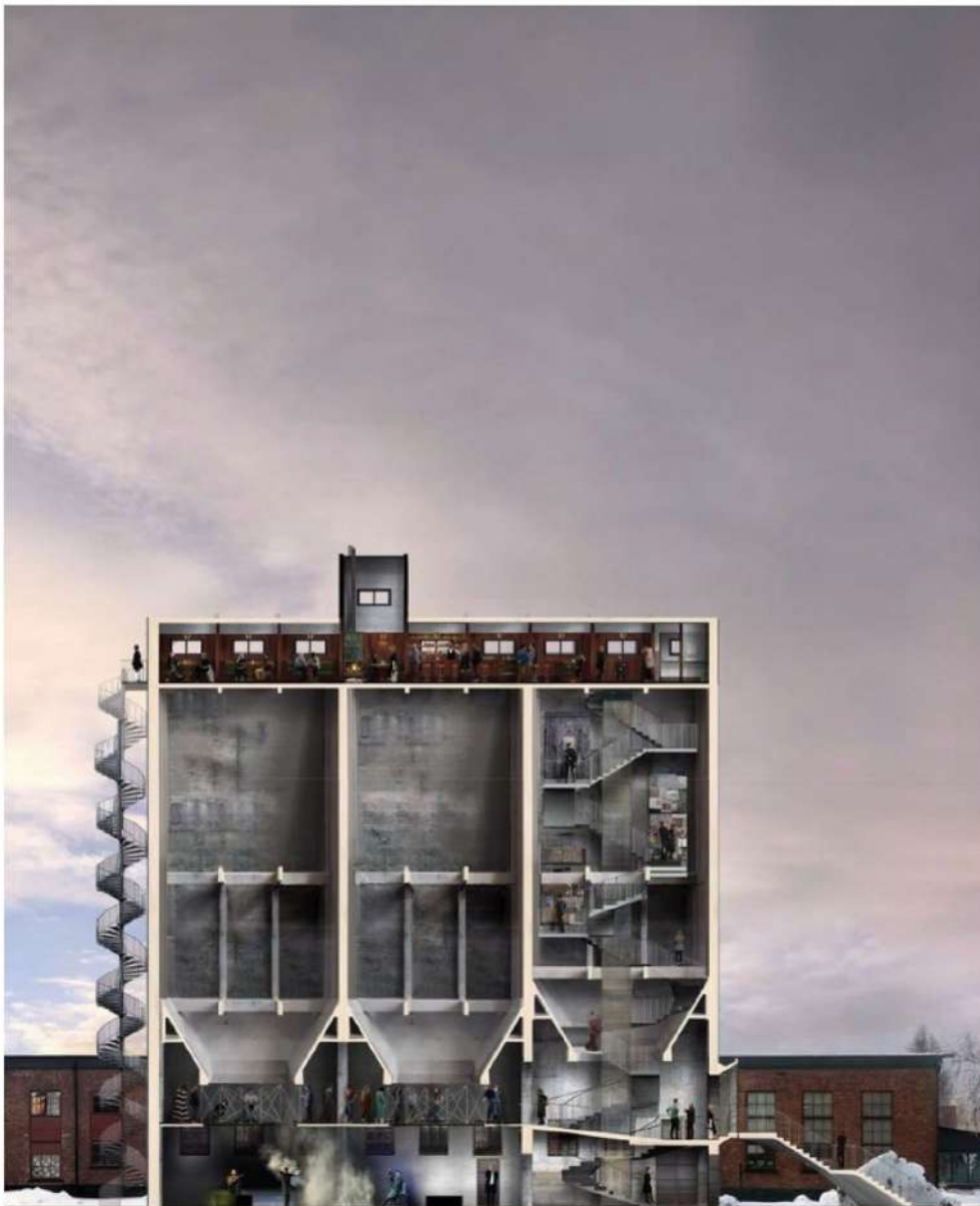
Cross-section of what Aaltosiilo could look like in the future. The building's original purpose of use is to be preserved in its structures. Visitors follow the same route as the wood chips in the building used to go.
