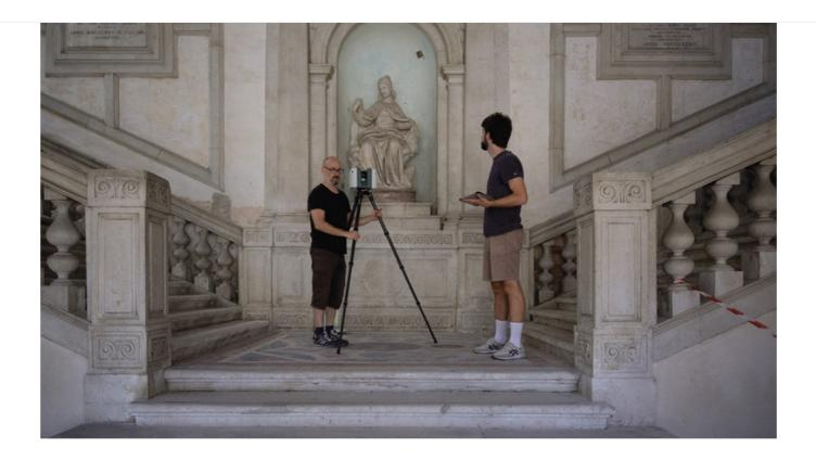
The first phase of the project ARCHiVe involved recording the Basilica of San Giorgio Maggiore, a 16th-century church designed by Andrea Palladio, using LiDAR scanning (using a Leica RTC360) and ground-based photogrammetry (using a Sony A7Riv camera). For the first days, the group recorded the interior of the Palladian church, the apse, and the inside of the bell tower, while the following days were dedicated to the exterior of the church and the crypt.
