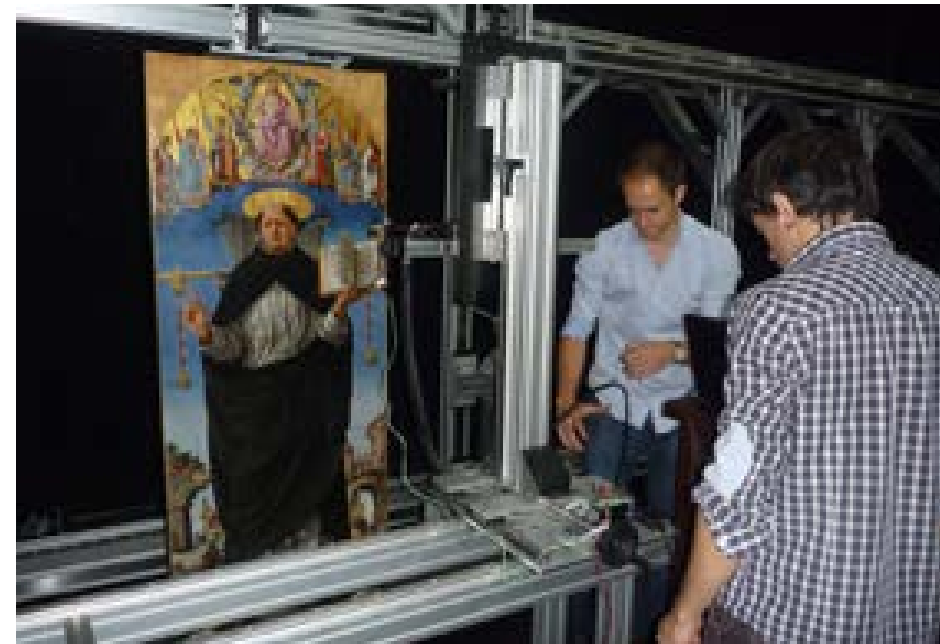
4a-c The surfaces of the paintings that make up the Polittico Griffoni being scanned in three dimensions using the Lucida scanner designed by Manuel Franquelo. Data is stored as raw black-and-white video that can be processed into three-dimensional files at increasingly high resolution in the future.
