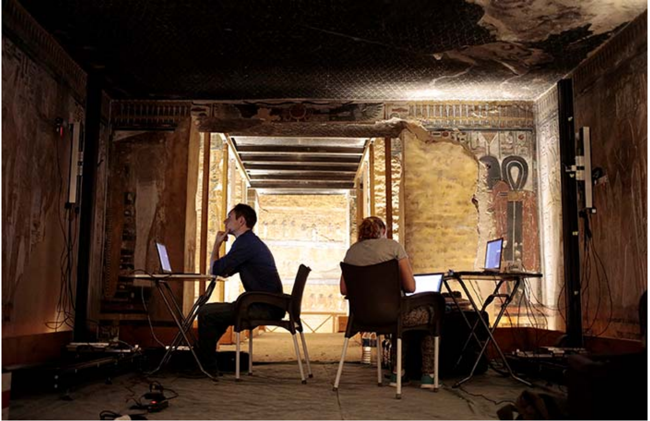
Carlos Bayod and Aliaa Ismail from Factum Arte scanning the Tomb of Seti I with the Lucida 3D scanner. Image © Gabriel Scarpa
