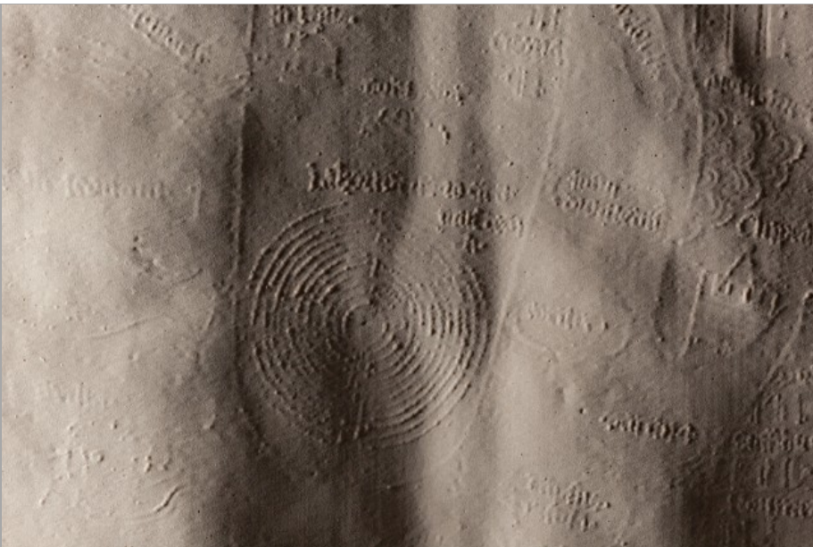
Detail of the texture of the routed sample of Hereford Mappa Mundi's 3D information. All marks of the map's texture were captured and reproduced.
