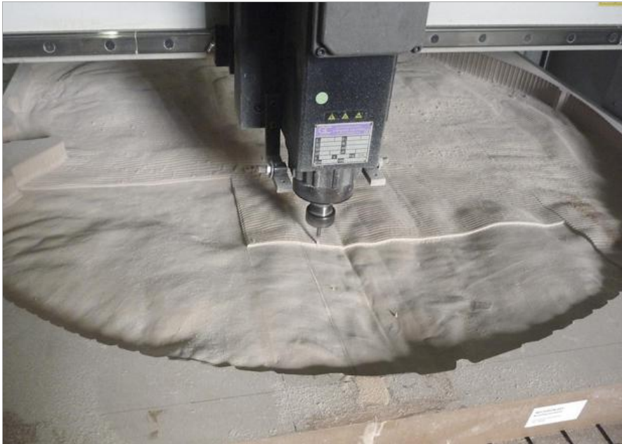
Process of routing the 3D information of the Hereford Mappa Mundi at 1:1 scale in Factum Arte's workshops in Madrid.
