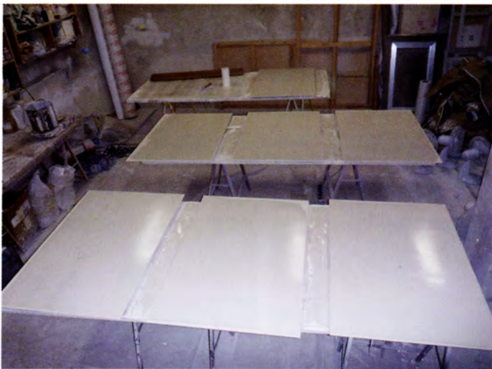
Fig 5: Gesso-covered aluminium, the substrate created in-house for use with the flatbed digital pigment printer.
