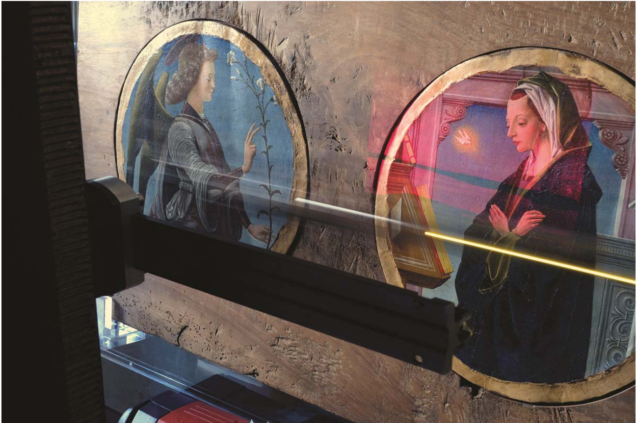
Factum Arte's Lucida 3D scanner recording works by Francesco del Cossa
