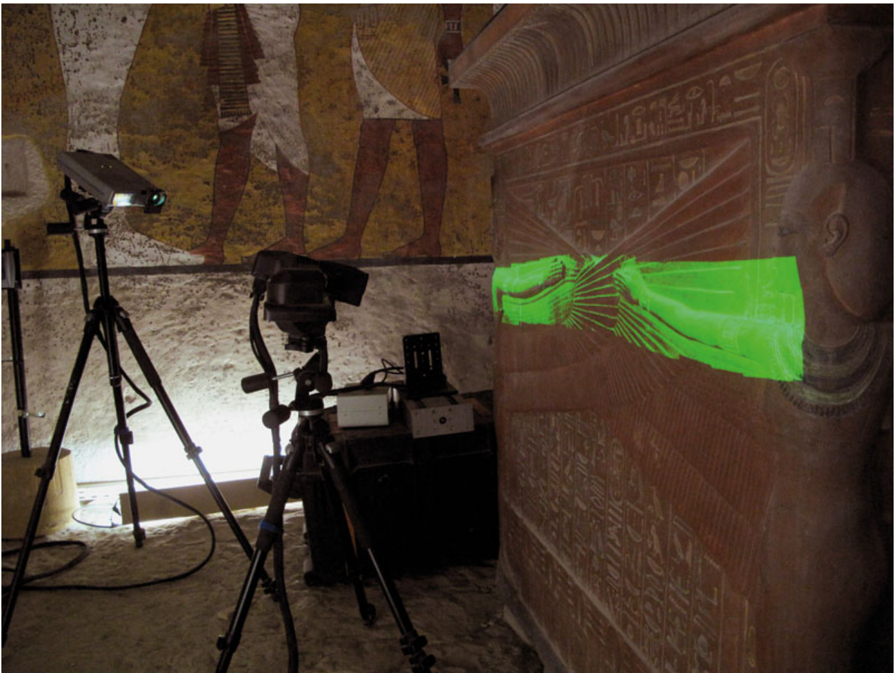
The Sidio Pro Scanner (White light scanner) during the recording of the sarcophagus in the Tomb of Tutankhamun, spring 2009 © Factum Arte
