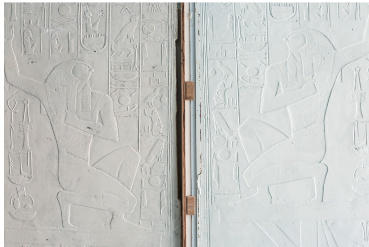
Océ 3D printing as a mould (right) from which the plaster cast is taken (left).
