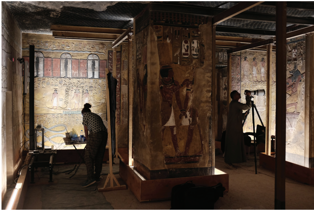
3D recording with the Lucida Laser Scanner on the left, and panoramic colour recording on the right.
