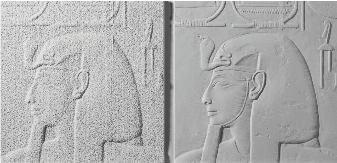
Comparison between the maximum resolution possible with the Faro LiDAR scanner (left) and a normal recording with the Lucida Laser Scanner (right). The file preparation and CNC strategy are constant.
