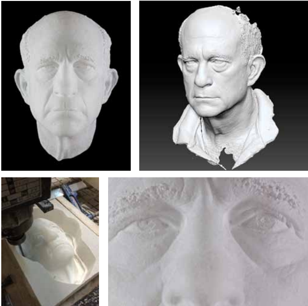
Portrait of Daniel Wolf in alabaster, 2015. Data from facial 3D scanner and routing process.
