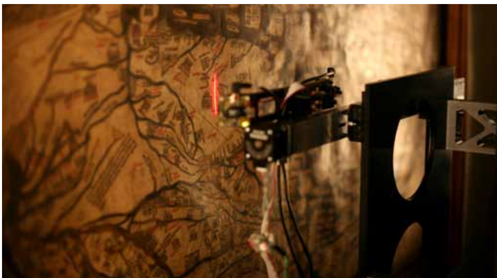
Top: Facsimile of the Tomb of Tutankhamun, Luxor. Bottom: Scanning process of the Hereford Mappa Mundi with the Lucida scanner developed by Manuel Franquelo and Factum Arte.
