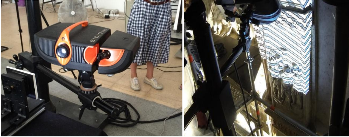
Left: The Nub 3D SIDIO scanner during calibration Right: The SIDIO scanning one of the pilasters of the left door on the façade of the Basilica of San Petronio, Bologna
