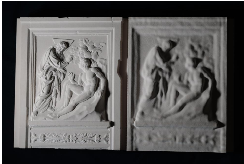
A routed sample from the façade of the Basilica of San Petronio in Bologna illustrating the difference in resolution and accuracy between close-range and long-medium range scanning – in this case the NUB3D SIDIO (left) and the Faro Focus 3D X330 (right).
