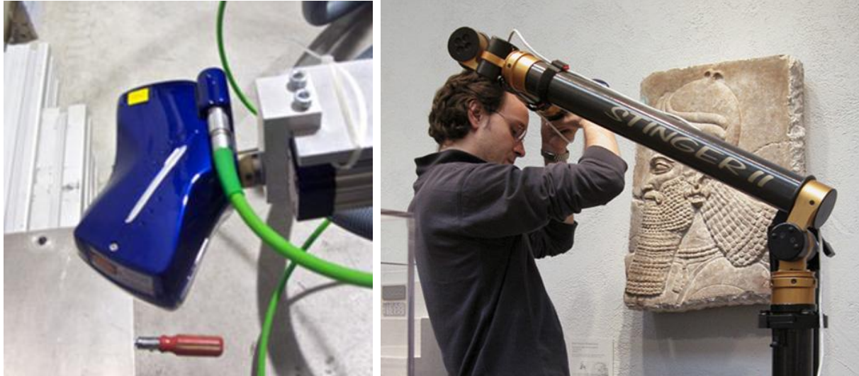
Left: The Kreon Zephyr 50 3D scanner head mounted on a robot Right: Gabriel Scarpa using the Kreon system (Cimcore Stringer arm pictured) to scan the head of a winged genie 9 th C BC relief from Harvard's Arthur M. Sackler Museum
