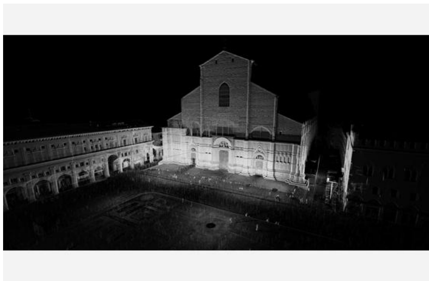
Visualization of Bologna's Piazza Maggiore and the facade of the Basilica recorded with FARO Focus 3D X 330 ©The Basilica of San Petronio
