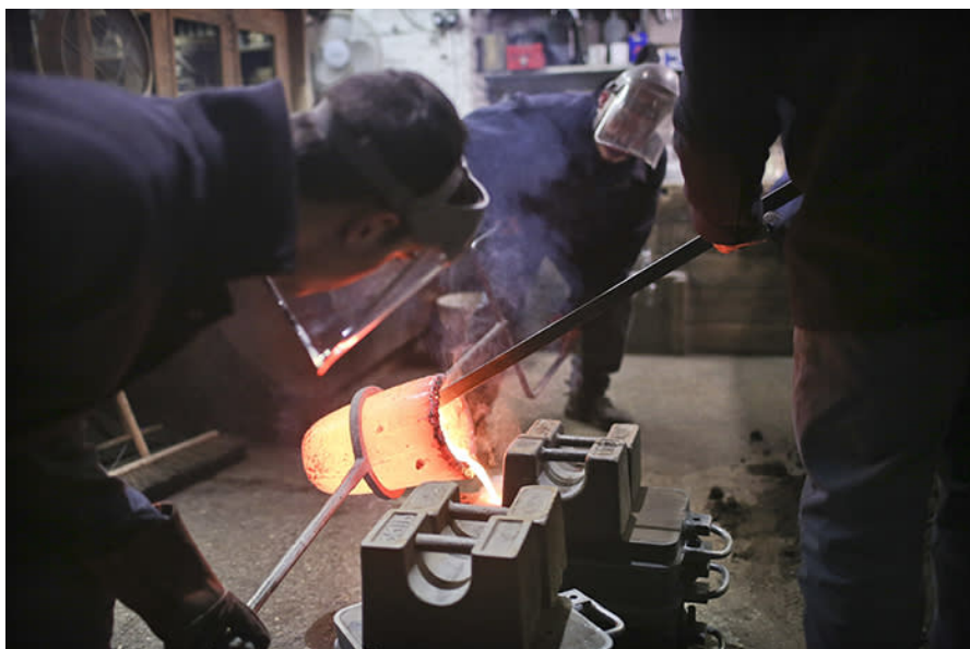
Pouring molten metal at the bell foundry © Charlie Bibby
