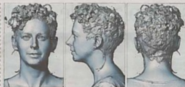
The scanner's eight cameras take four seconds to take pictures from all angles
