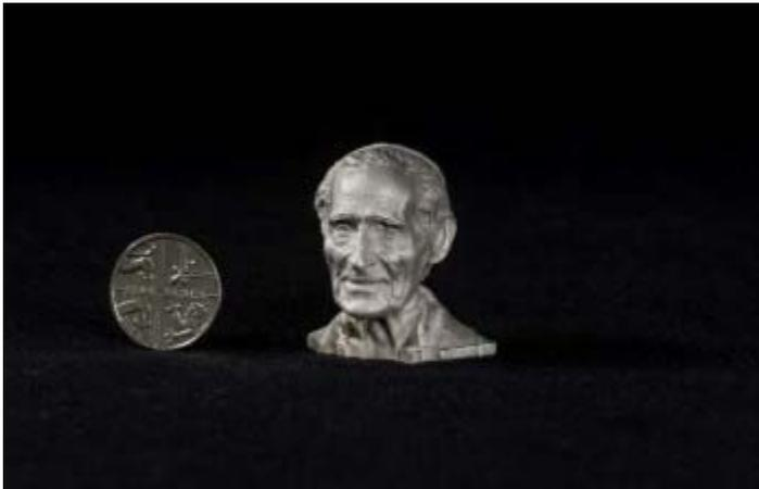
A sterling silver cast produced from a wax 3D print still retains incredible detail.
