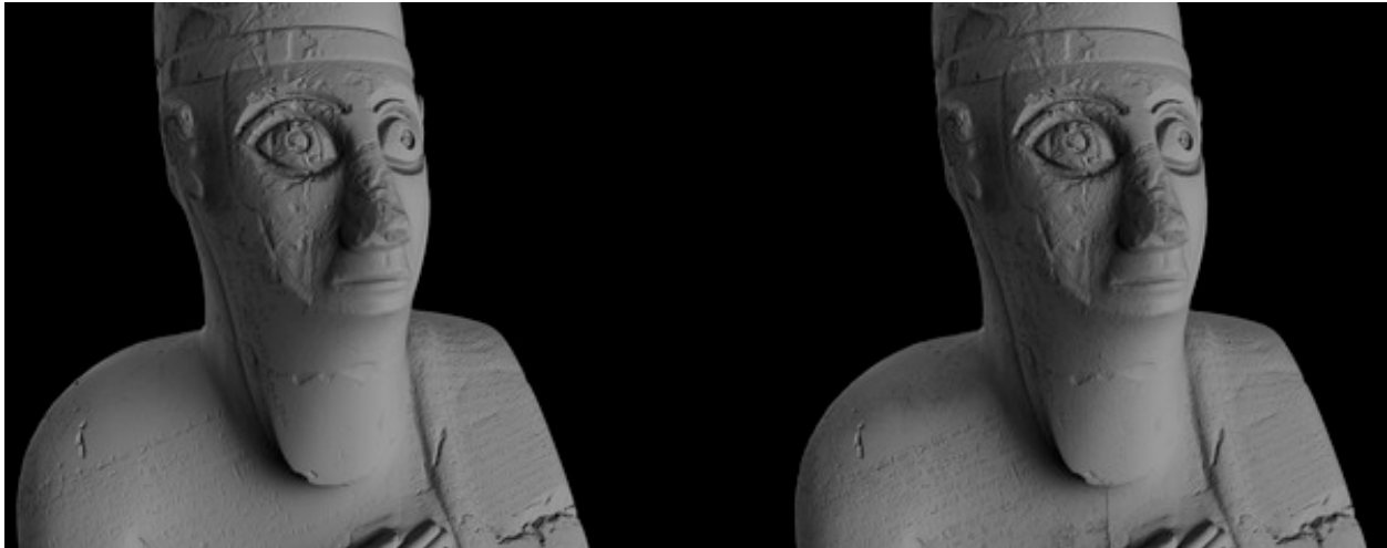
Three-dimensional models created using data recorded via white light scanning (left) and photogrammetry (right)
